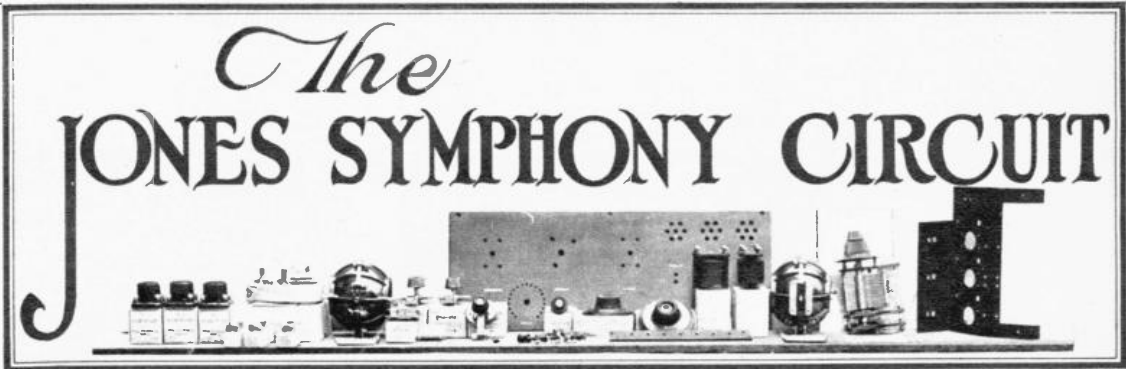
This is the complete lay-out of apparatus, panel, bracket and everything just as it comes ready for assembling.
